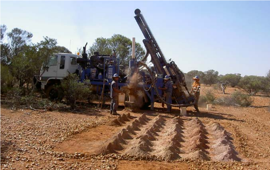
Figure 6: Aircore drilling and sampling operation.
