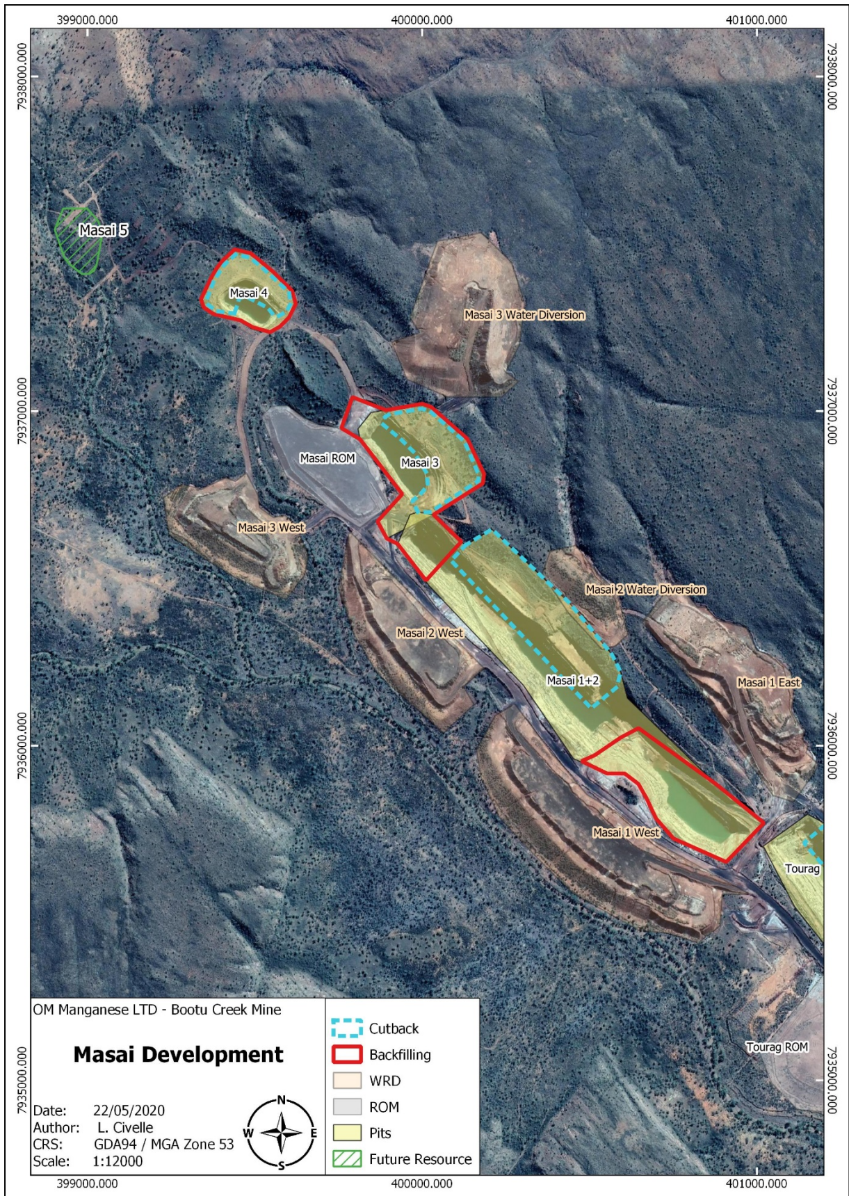
Figure 13: Mine features and plans for the development of the Masai ore body at the BCMM.
