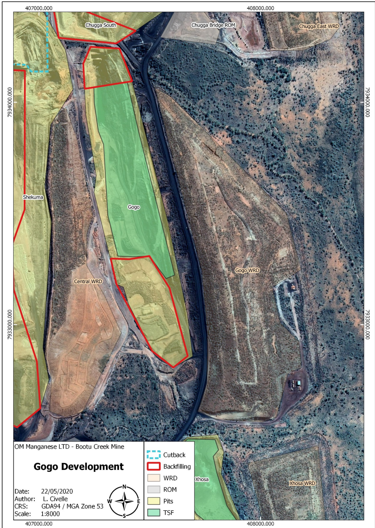
Figure 24: GoGo open cut pit and associated waste rock landforms.
