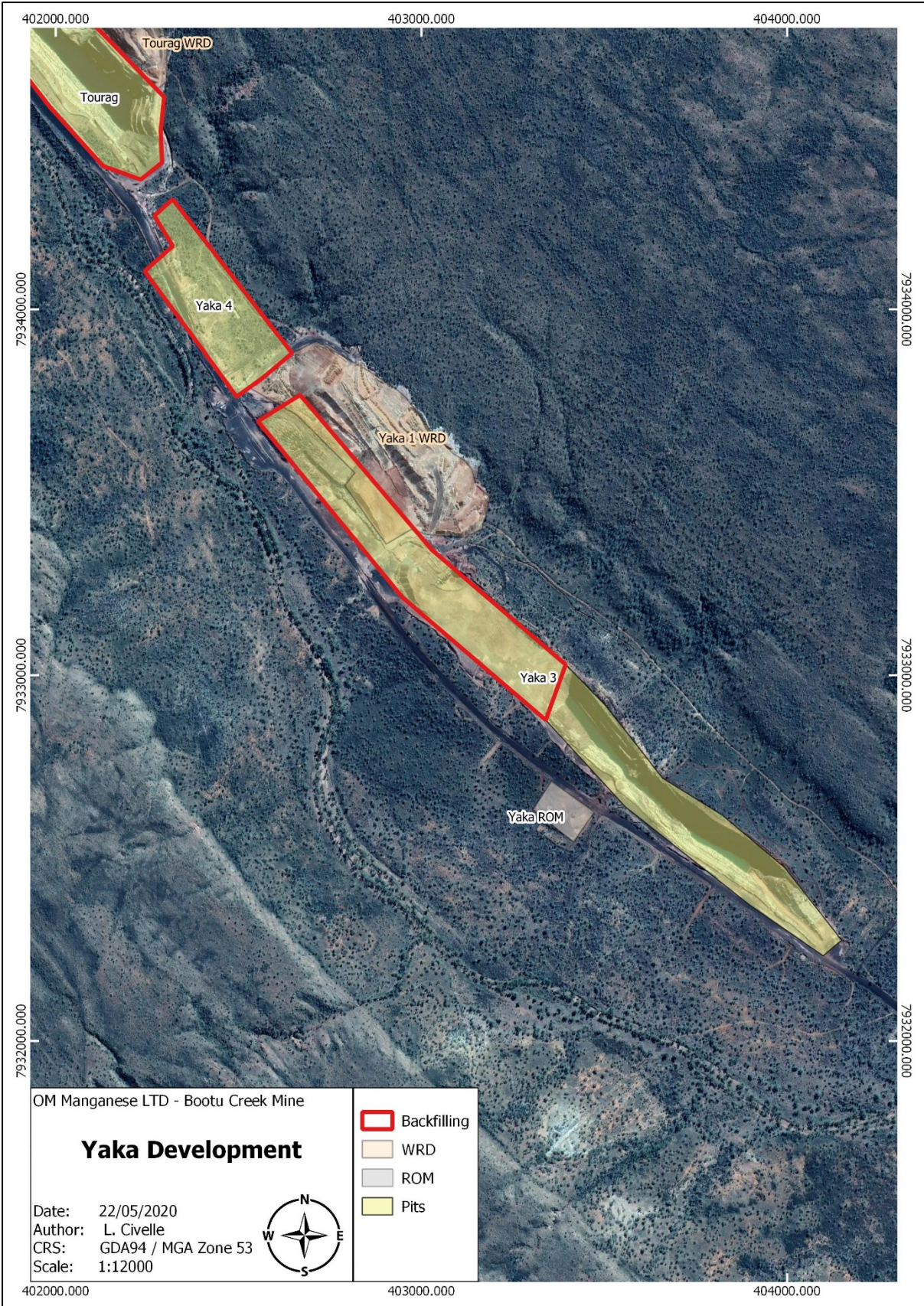
Figure 20: Open cut pits and associated waste rock landforms of the Yaka development.
